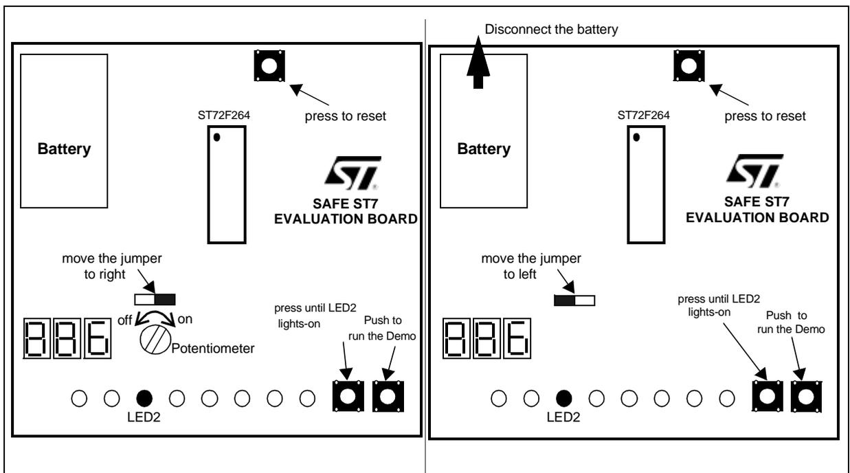
In case of power drop, and before going into reset state, the AVD interrupt will save the last displayed value in the external EEPROM (M24C08) using the I<sup>2</sup>C protocol. On power-on, the software checks if the last reset was made by the LVD, if this is the case, it downloads the previously saved value from the external EEPROM to RAM memory in order to resume counting as normal.
