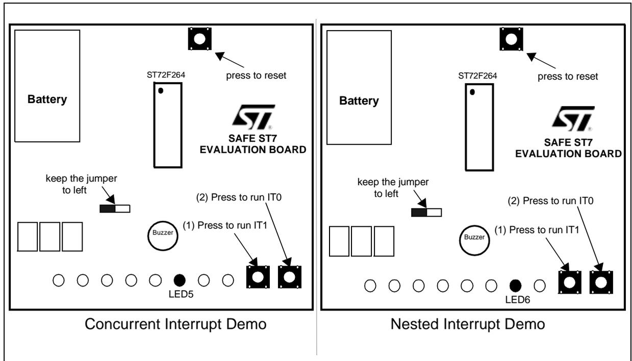
As shown in [Figure 17](#) this demo is divided into two parts: The first one runs concurrent interrupts while the second uses nested interrupts.
