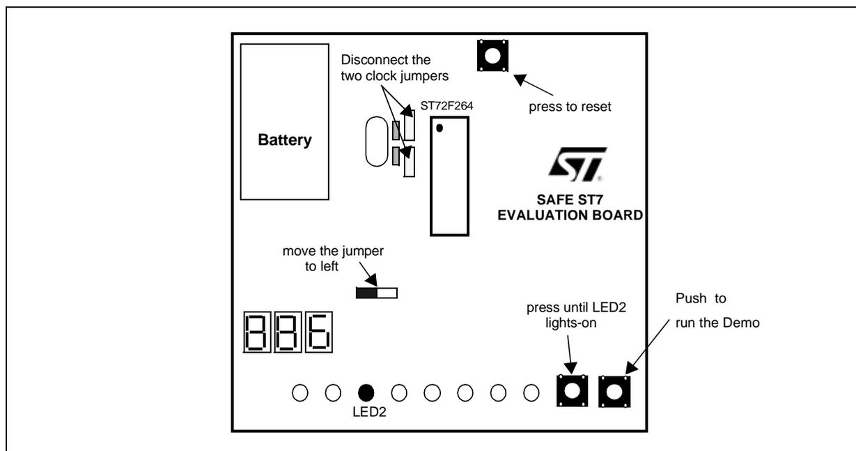
If the clock signal disappears, which you can provoke by disconnecting the two jumpers as shown in [Figure 13](#), the safe oscillator delivers a low frequency clock signal (around 3MHz) for a safe oscillator period which allows the ST7 to save any critical data or perform any kind of emergency operations while the CPU is still running.
