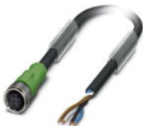
Sensor/actuator cable, 4-position, PUR, black-gray RAL 7021, free cable end, on Socket straight M12, A-coded, cable length: 6 m
