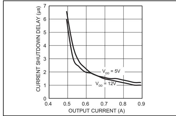
**FIGURE 2-4:** Current Shutdown Delay vs. Output Current.
