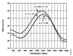
Figure 14. Noise vs. Frequency
