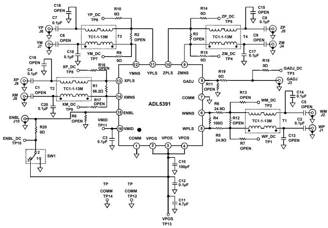
Figure 23. ADL5391-EVALZ Evaluation Board Schematic
