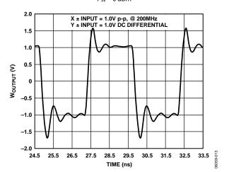
Figure 8. Large Signal Pulse Response
