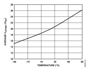
Figure 11. X(Y) Offset Drift vs. Temperature
