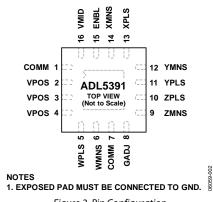
Figure 2. Pin Configuration
