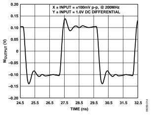
Figure 9. Small Signal Pulse Response
