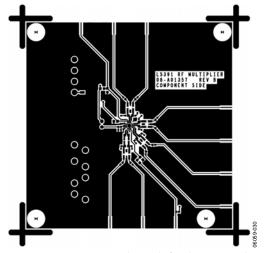
Figure 24. Component Side Metal of Evaluation Board
