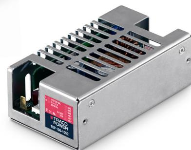
The new TOP-100 Series AC/DC Power Supplies feature the highest power rating in the industry standard 2.0" x 4.0" (50.8 x 101.6 mm) footprint. They can supply up to 100 W output power with convection cooling over an industrial operating temperature range of -25°C to +50°C. This performance could be realized by a state of the art design providing an extremely high efficiency of >90 % which eliminates the need for a dedicated power supply cooling fan.
