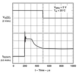
Figure 10. 4- $\Omega$  Load Connected to Enabled Device
