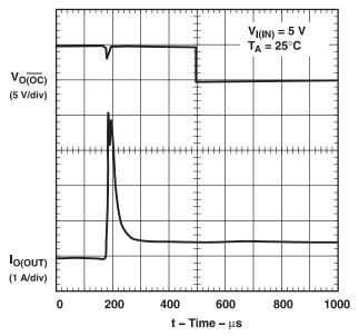
Figure 11.  $1-\Omega$  Load Connected to Enabled Device
