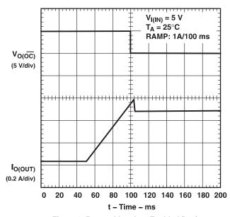
Figure 8. Ramped Load on Enabled Device
