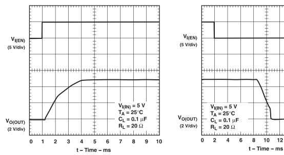
Figure 2. Turnon Delay and Rise Time With  $0.1-\mu F$  Load
