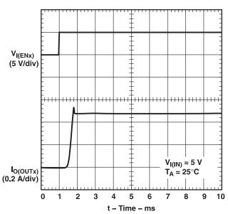
Figure 6. TPS2090, Short-Circuit Current, Device Enabled Into Short
