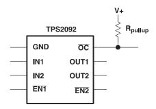
Figure 25. Typical Circuit for OC Pin
