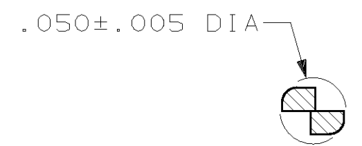
SECTION A-A SCALE 10:1 10 PLACES
