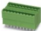
PCB headers, nominal current: 10 A, rated voltage (III/2): 320 V, nominal cross section: 2.5 mm<sup>2</sup>, number of positions: 8, pitch: 5 mm, color: green, contact surface: Tin, mounting: Wave soldering, pin layout: Linear pinning, solder pin [P]: 3.9 mm, In combination with MVSTB or FKCV plug components, both an MVSTBW (or FKCVW) and an MVSTBR plug (or FKCVR) must be used. Combination with TMSTBP plug components is not possible!
