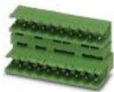
PCB headers, nominal current: 10 A, rated voltage (III/2): 320 V, nominal cross section: 2.5 mm<sup>2</sup>, number of positions: 8, pitch: 5 mm, color: green, contact surface: Tin, mounting: Wave soldering, pin layout: Linear pinning, solder pin [P]: 3.2 mm, Can be aligned! Mounting flange: Order No. 1736771, 1736768. In combination with MVSTB or FKCV plug components, both an MVSTBW (or FKCVW) and an MVSTBR plug (or FKCVR) must be used. Combination with TMSTBP plug components is not possible!
