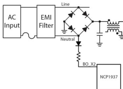
Figure 3. Brown-out and Line Voltage Detectors Configuration
