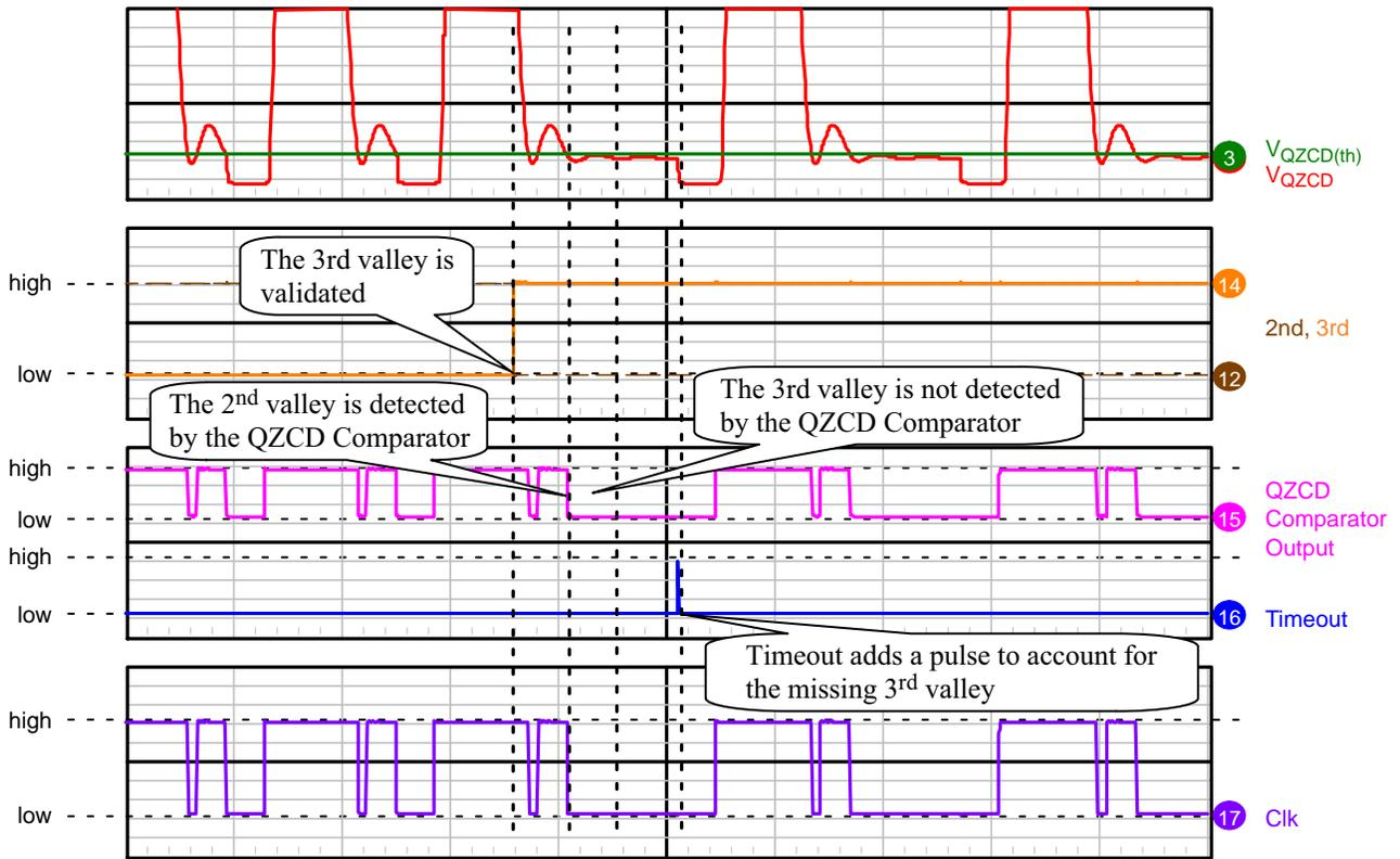
Figure 22. Timeout Operation with a Missing 3<sup>rd</sup> Valley
