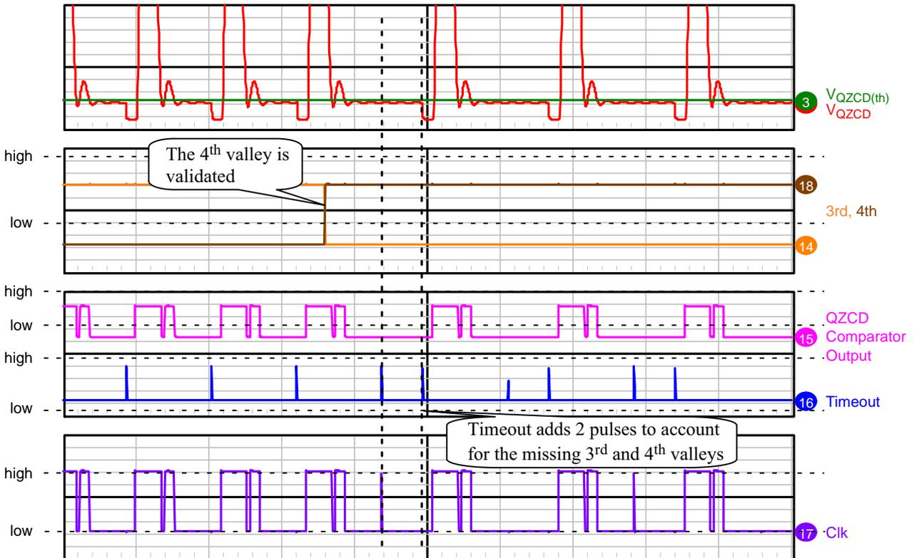
Figure 23. Timeout Operation with Missing 3<sup>rd</sup> and 4<sup>th</sup> Valleys
