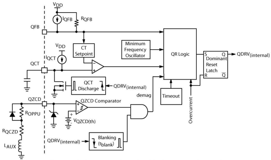
Figure 13. Valley Lockout Detection Circuitry Internal Schematic
