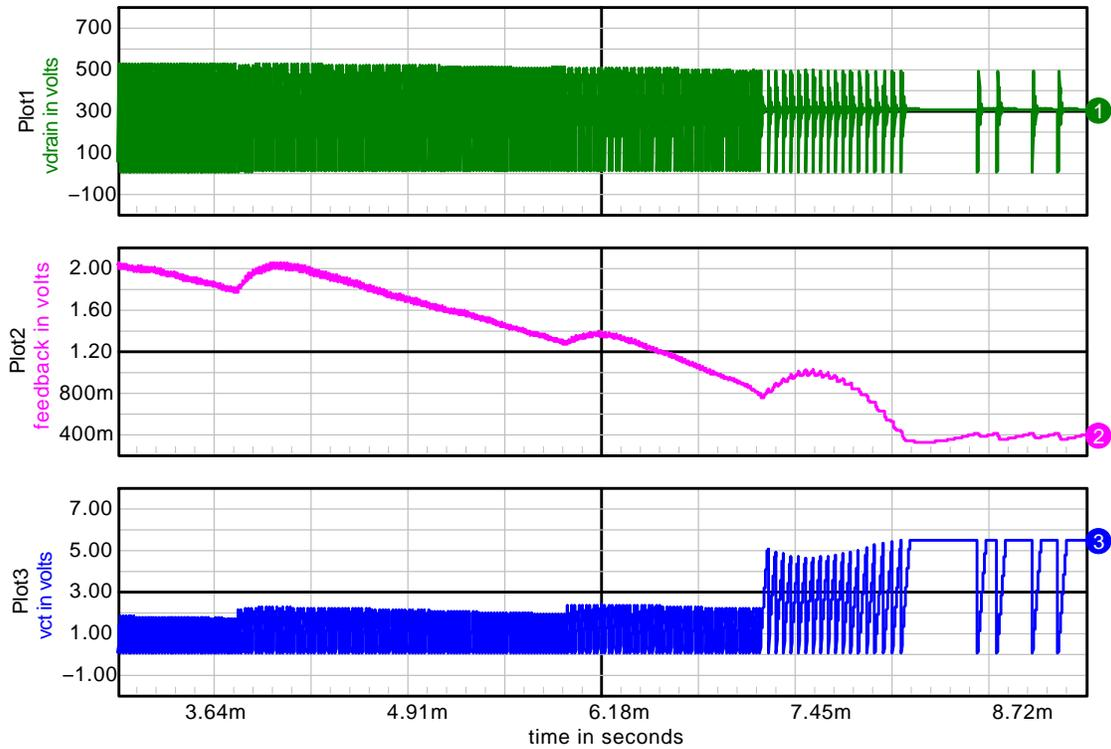
Figure 16. Operating Mode Transitions between 2<sup>nd</sup> to 3<sup>rd</sup>, 3<sup>rd</sup> to 4<sup>th</sup> and 4<sup>th</sup> Valley to VCO Mode
