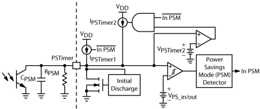
Figure 7. NCP1937 Power Savings Mode Control Block Diagram
