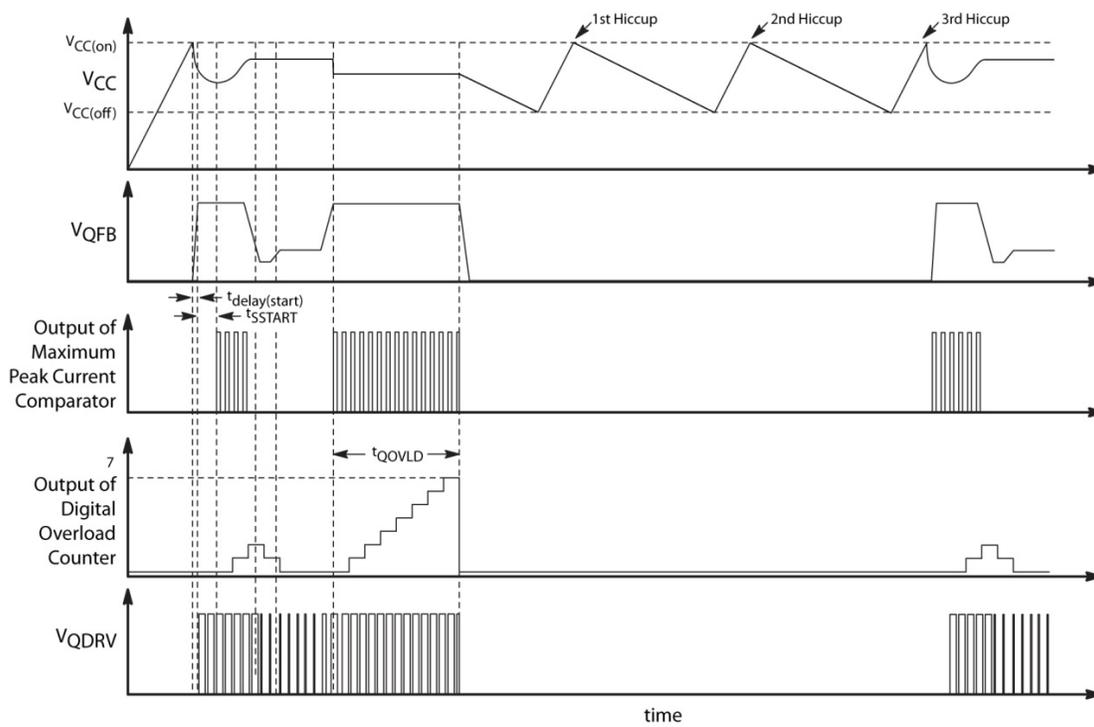
**Figure 26. Auto-recovery Overload Operation**
