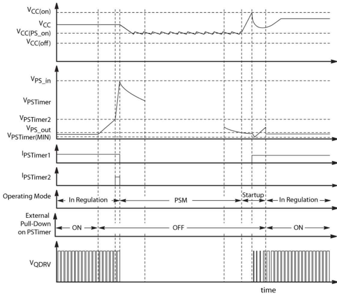
Figure 8. NCP1937 Power Savings Mode Operating Waveforms
