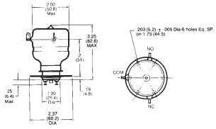
**Product Specifications for** H-19 and H-17 Contact Arrangement — H-19 — DPDT H-17 — SPDT Contact Form — H-19 — 2C H-17 — C Test Voltage, DC or 60 Hz (Peak) -H-19 — 25 kV H-17 — 30 kV Rated Operating Voltage (Peak) -DC or 60 Hz — H-19 — 20 kV H-17 - 25 kV 2.5 MHz - H-19 - 15 kV H-17 - 20 kV 16 MHz — H-19 — 10 kV H-17 — 15 kV 32 MHz — H-19 — 7 kV H-17 — 12 kV Continuous Carry Current, Max. -DC or 60 Hz - 30 A 2.5 MHz — H-19 — 18 A H-17 — 16 A
