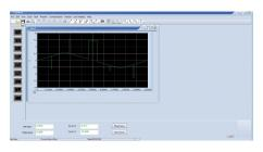
The provided waveform editing software can be used to create point-by-point arbitrary waveforms via freehand or waveform math functions. A standard USBTMC-compliant USB device port on the rear panel allows users to easily interface with a PC to load these arbitrary waveforms into the instrument.
