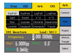
All models in the 4050 series have non-volatile memory to create, store, and recall up to 10 different arbitrary waveforms of up to 16,000 points each. Users can also output any of the 48 built-in predefined arbitrary waveforms.
