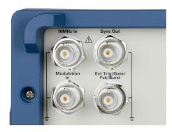
Use the external 10 MHz clock input to synchronize your signals to a master time base. The Sync output generates a TTL pulse for synchronization to a channel's frequency. An external trigger connector is also available for inputting or outputting trigger signals.
