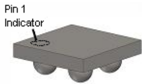
Figure 3. 1 x 1mm WLCSP Bumps Facing Down
