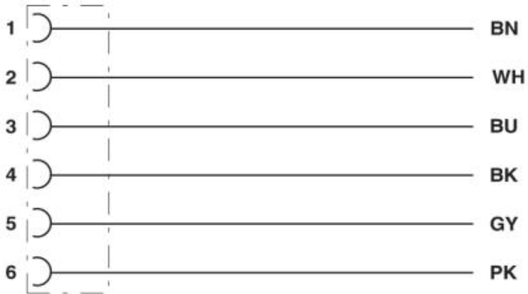
Contact assignment of M8 socket
