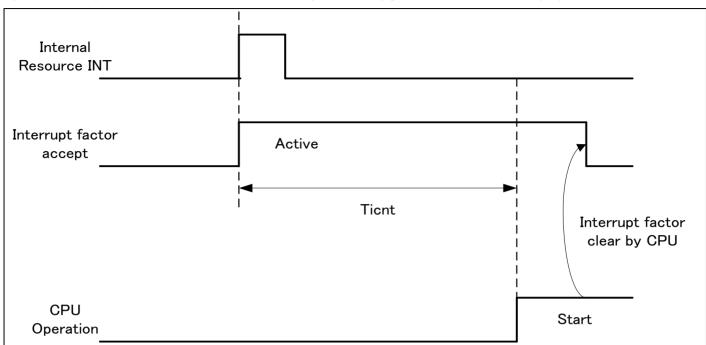
Operation example of return from Low-Power consumption mode (by internal resource interrupt<sup>\*1</sup>)
