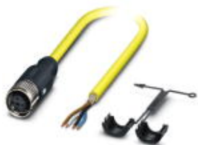
Sensor/actuator cable, 4-position, PVC, yellow, shielded, free cable end, on Socket straight M12 SPEEDCON, A-coded, cable length: 2 m
