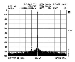
Figure 5. AD9956 DAC Performance: 400 MSPS Clock, 40 MHz F<sub>OUT</sub>, 1 MHz Span
