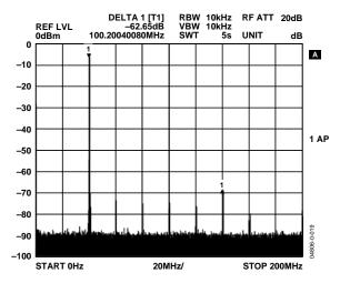
Figure 8. AD9956 DAC Performance: 400 MSPS Clock, 40 MHz F<sub>OUT</sub>, 200 MHz Span
