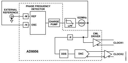
Figure 25. Optical Networking Clock
