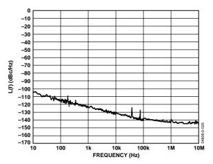
Figure 14. AD9956 DDS/DAC Residual Phase Noise 400 MHz Clock, 103 MHz Output
