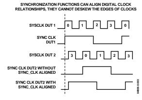
Figure 28. Synchronization Functions: Capabilities and Limitations
