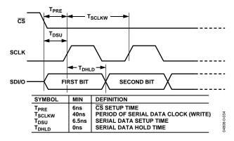
Figure 33. Timing Diagram for Data Write to AD9956
