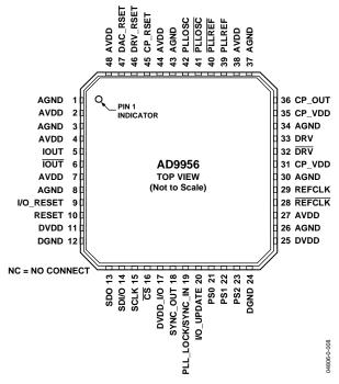
Figure 3. 48-Lead LFCSP Pin Configuration
