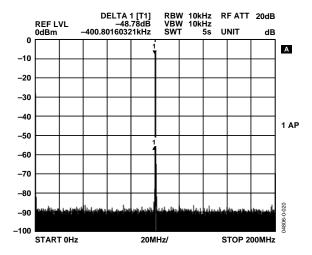
Figure 9. AD9956 DAC Performance: 400 MSPS Clock, 100 MHz F<sub>OUT</sub>, 200 MHz Span
