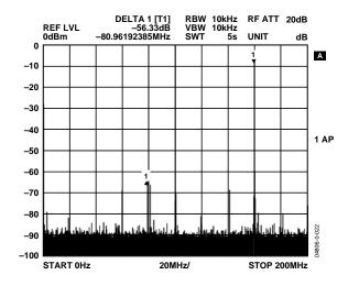
Figure 13. AD9956 DAC Performance: 400 MSPS Clock, 160 MHz F<sub>OUT</sub>, 200 MHz Span
