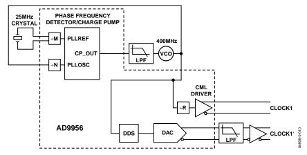
Figure 22. Dual-Clock Configuration
