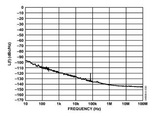
Figure 19. RF Divider and CML Driver Residual Phase Noise (2488 MHz In, 622 MHz Out)
