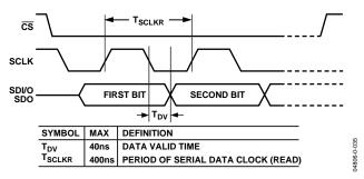
Figure 34. Timing Diagram for Data Read to AD9956
