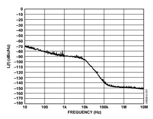
Figure 20. Total System Phase Noise for 105 MHz Converter Clock
