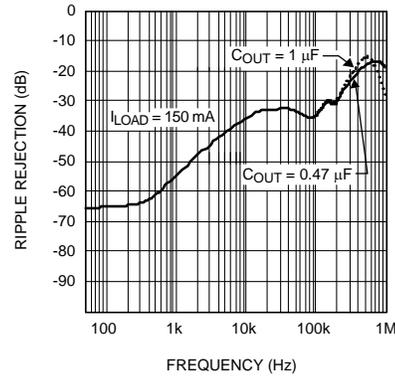
Figure 10. Power Supply Rejection Ratio
