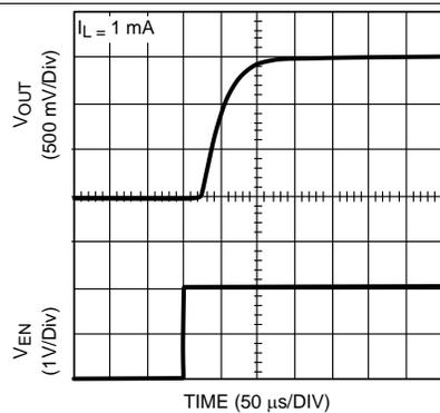
Figure 11. Enable Start-Up Time
