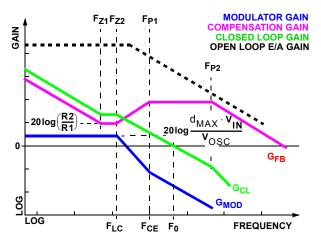
FIGURE 10. ASYMPTOTIC BODE PLOT OF CONVERTER GAIN
