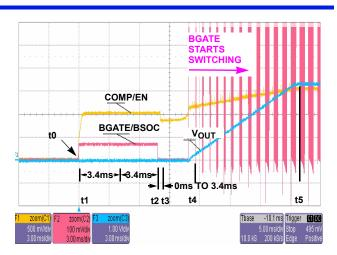
FIGURE 2. BGATE/BSOC AND SOFT-START OPERATION
