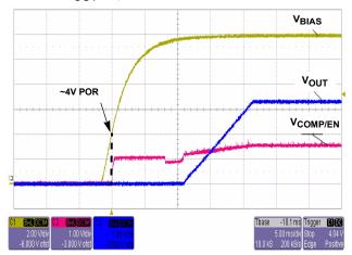
FIGURE 1. POR AND SOFT-START OPERATION
