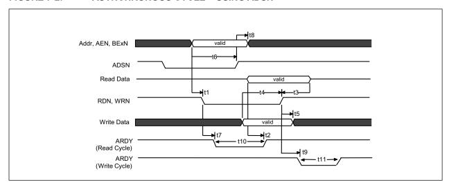
TABLE 7-2: ASYNCHRONOUS CYCLE USING ADSN TIMING PARAMETERS
