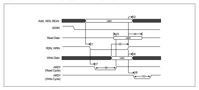
TABLE 7-1: ASYNCHRONOUS CYCLE (ADSN = 0) TIMING PARAMETERS
