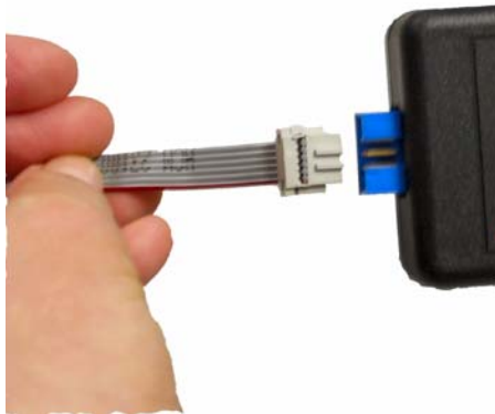
Figure 2. Connecting the Six-Conductor Ribbon Cable to the Serial or USB Smart Cable
