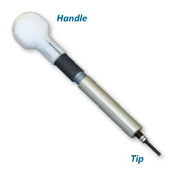
Check for properly seated contacts with this spring-loaded tester. Apply the tool tip to the mating end of a contact. Push on the handle until the spring compresses to the recommended force. A visual indicator shows full compression. The contact is properly retained if it is not displaced.
