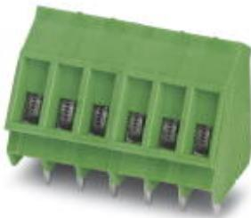
PCB terminal block, Nominal current: 24 A, Nom. voltage: 400 V, Pitch: 5 mm, Number of positions: 12, Connection method: Screw connection with tension sleeve, Mounting: Wave soldering, Conductor/PCB connection direction: 55 °, Color: green, The article can be aligned to create different nos. of positions!
