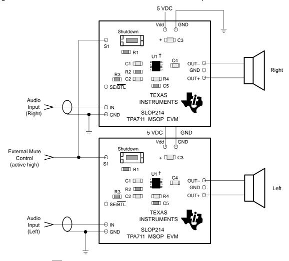
**Note:** The (SE/ $\overline{BTL}$ ) EVM pin is pulled to GND through a 20-k $\Omega$  resistor on the module.
