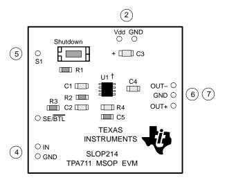
† Due to the very small size of the MSOP IC package, the standard part number TPA711 is replaced with the code TIABB
