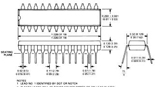
LEAD NO 1 IDENTIFIED BY DOT OR NOTCH. PLASTIC LEADS WILL BE EITHER SOLDER DIPPED OR TIN LEAD PLATED IN ACCORDANCE WITH MIL-M-38510 REQUIREMENTS
