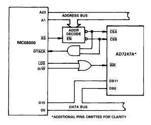
Figure 12. AD7247A to MC68000 Interface
