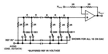
Figure 2. D/A Simplified Circuit Diagram
