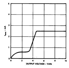
Single Supply Sink Current vs. Output Voltage
