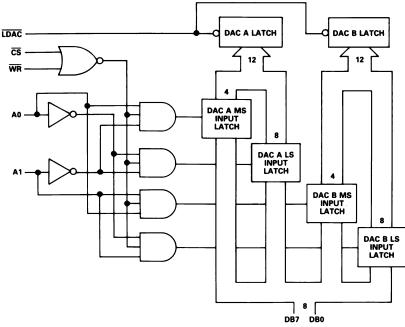
Figure 6. AD7237A Input Control Logic
