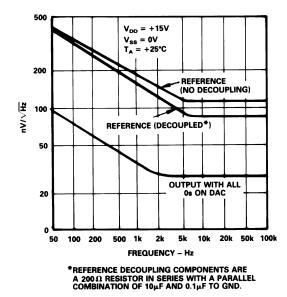
Noise Spectral Density vs. Frequency
