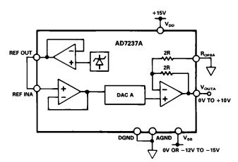
Figure 8. Unipolar (0 to +10 V) Configuration
