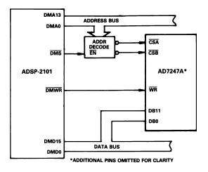
Figure 10. AD7247A to ADSP-2101 Interface
