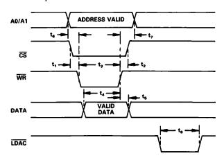
Figure 7. AD7237A Write Cycle Timing Diagram
