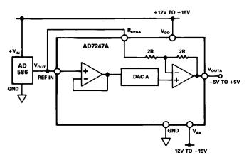
Figure 9. Bipolar Configuration
