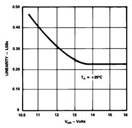
Linearity vs. Power Supply Voltage
