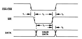
Figure 5. AD7247A Write Cycle Timing Diagram
