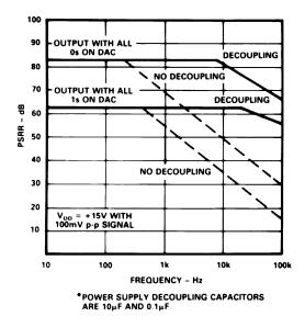
Power Supply Rejection Ratio vs. Frequency
