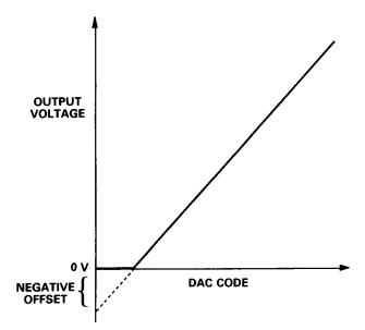
Figure 1. Effect of Negative Offset (Single Supply)
