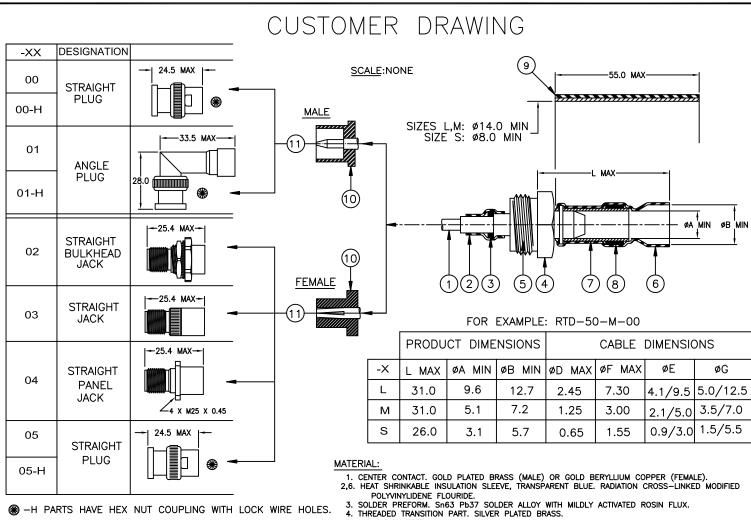
⊕ -H PARTS HAVE HEX NUT COUPLING WITH LOCK WIRE HOLES.
