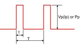
Where:Vp: Pulse limiting voltage (V)
