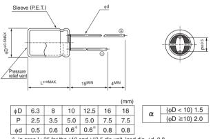
$\%\,$  In case L>25 for the  $\phi10$  and  $\phi12.5$  dia unit, lead dia  $\,\phi d{=}0.8$
