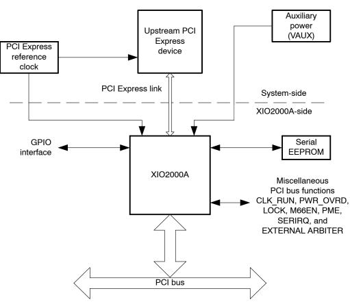
Figure 1. Typical System Integration
