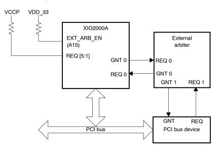
Figure 4. External Arbiter Connections
