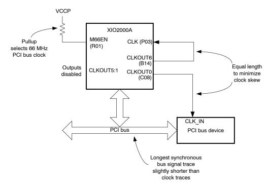
Figure 3. External PCI Bus Clock Feedback
