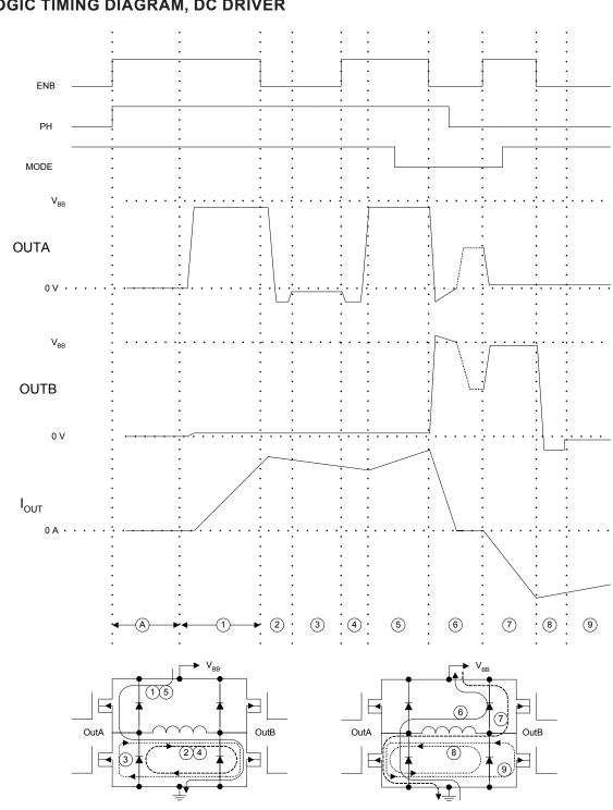
LOGIC TIMING DIAGRAM, DC DRIVER
