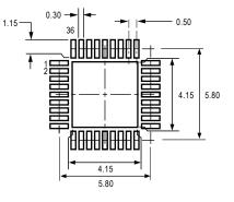
All dimensions nominal, not for tooling use (reference JEDEC MO-220VJJD-3, except pin count) Dimensions in millimeters Exact case and lead configuration at supplier discretion within limits shown
