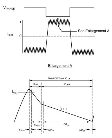
Figure 2. Mixed Decay Mode Operation
