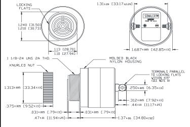
NOTE A: TERMINALS-0.32 BRASS TIN PLATED, TAPPED FOR #6-32 SCREW. TWO #6-32 NICKEL PLATED BRASS SCREWS INCLUDED. WILL ACCEPT 1/4\* OUICK CONNECT.
