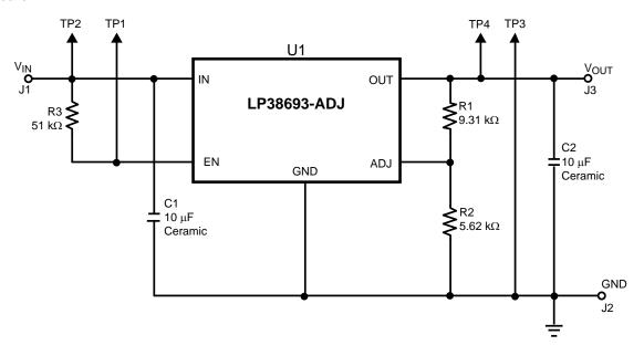
Figure 1. Evaluation Board Basic Application Circuit
