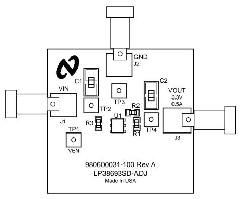
Figure 2. Evaluation Board Component Layout (Top View)
