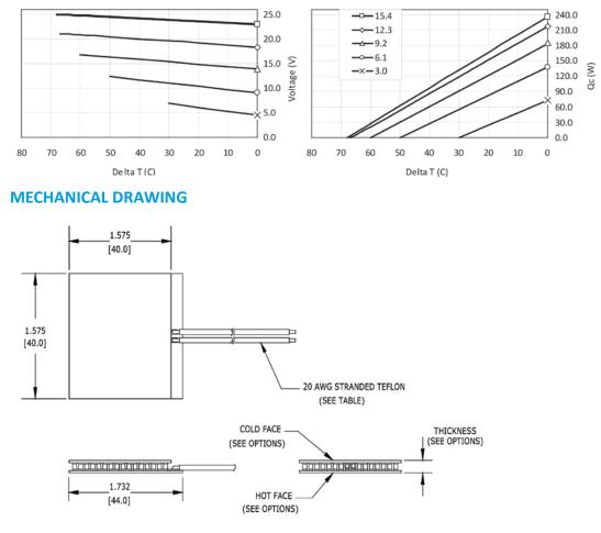
Ceramic material 96% Alumina ceramics Solder construction: 138°C BiSn
