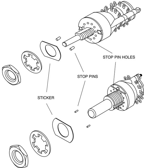
The adjustable stop Series 71 rotary switches allow you to change the number of positions per pole. Simply remove and relocate stop pins in the holes in the front of the switch. The pins are held in place by a self adhesive sticker which fits over the front plate.
