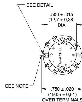
**Note:** Common location for a single pole per deck switch. For common location on multiple switches see circuit diagrams.
