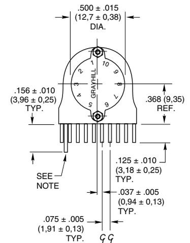
**Note:** Common location for a single pole per deck switch. For common location on two pole switches see circuit diagrams.
