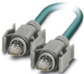
Assembled Ethernet cable, CAT5e, shielded, 4-pair, AWG 26 stranded (7-wire), line, RAL 5021 (water blue), RJ45/IP67 on RJ45/IP67, length: 2 m
