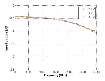
Figure 12. Insertion Loss @ 3.0V
