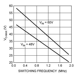
Figure 6. V<sub>OUT-MAX</sub> vs f<sub>sw</sub>
