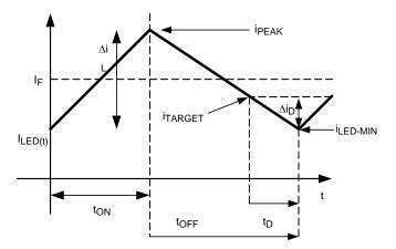
Figure 5. I<sub>SENSE</sub> Current Waveform
