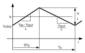
Figure 3. Buck Converter Inductor Current Waveform
