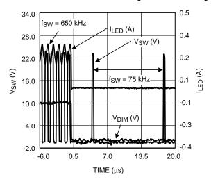
Figure 15. Improved Avg I<sub>LED</sub> Circuit + Fast Dimming
