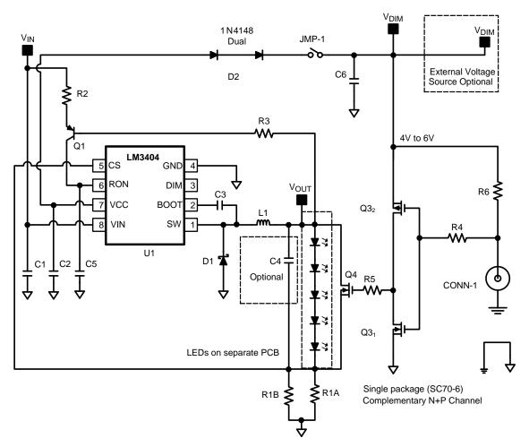
Figure 1. LM3402 / 04 Schematic
