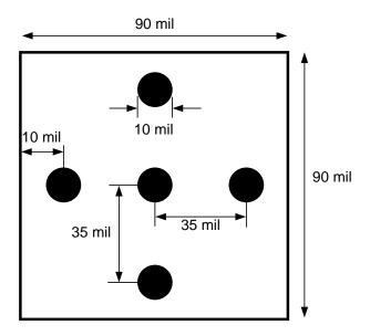
Figure 2. LM3402/04 PSOP Thermal PAD and Via Layout
