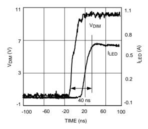
Figure 13. t<sub>D</sub> + t<sub>SU</sub> Graph
