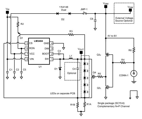
Figure 17.  $V_{IN}$  = 9V to 18V,  $I_{LED}$  = 700 mA, 3 x 3.4V White LED Strings ( $f_{SW} \approx 500$  kHz)
