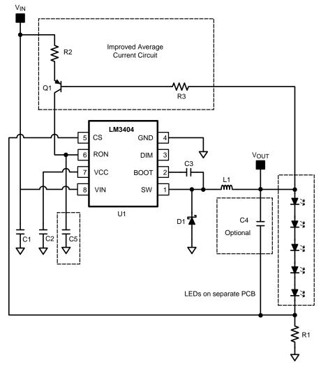
Figure 9. Improved Average LED Current Application Circuit
