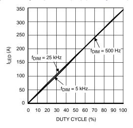
Figure 16. Linearity With Fast Dimming
