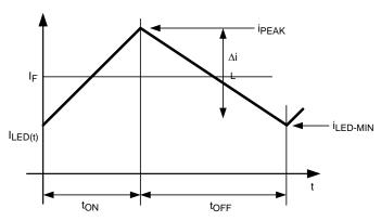
**Figure 8. Inductor Current Waveform**
