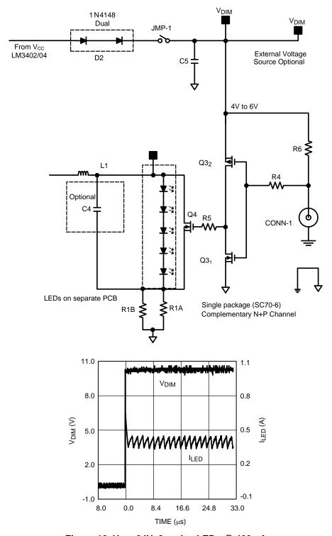
Figure 12.  $V_{IN}$  = 24V, 3 series LEDs @ 400mA
