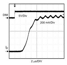
Figure 11. t<sub>D</sub> and t<sub>SU</sub> (DIM Pin)
