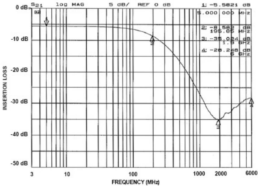
Figure 8. Insertion Loss vs. Frequency (Filter 8 Input – Pin 8 to Pin 9)
