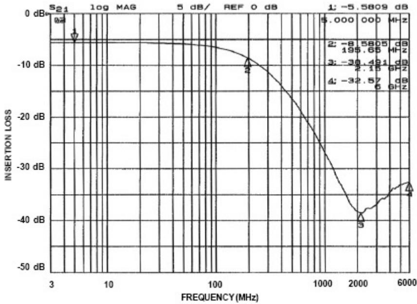
Figure 3. Insertion Loss vs. Frequency (Filter 3 Input – Pin 3 to Pin 14)
