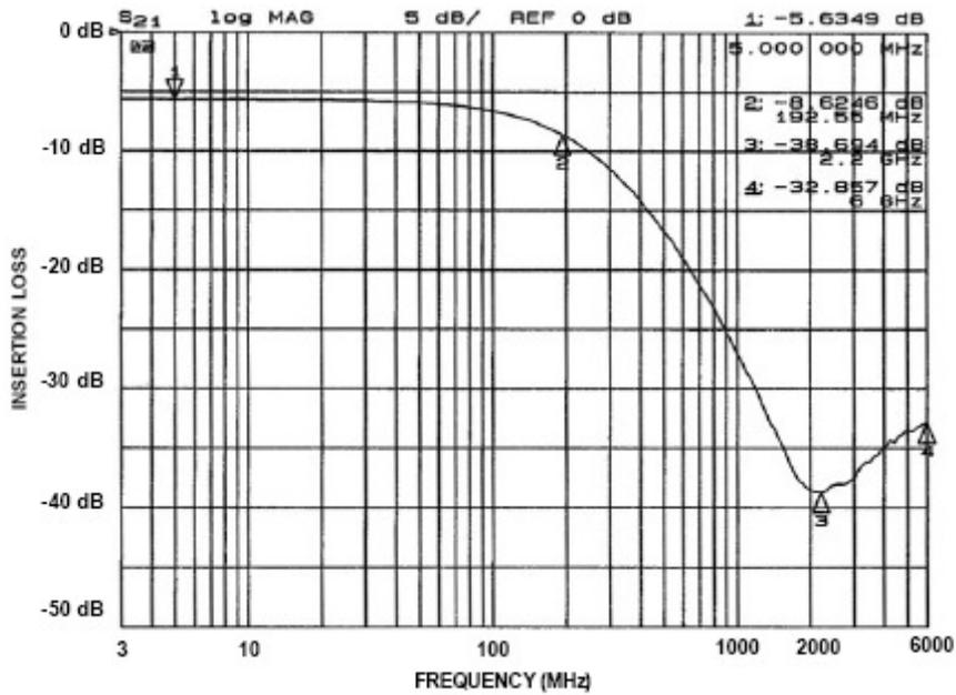
Figure 2. Insertion Loss vs. Frequency (Filter 2 Input – Pin 2 to Pin 15)
