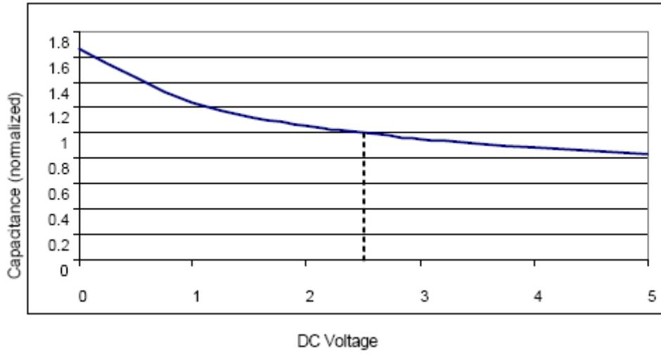
Figure 9. Filter Capacitance vs. Input Voltage
