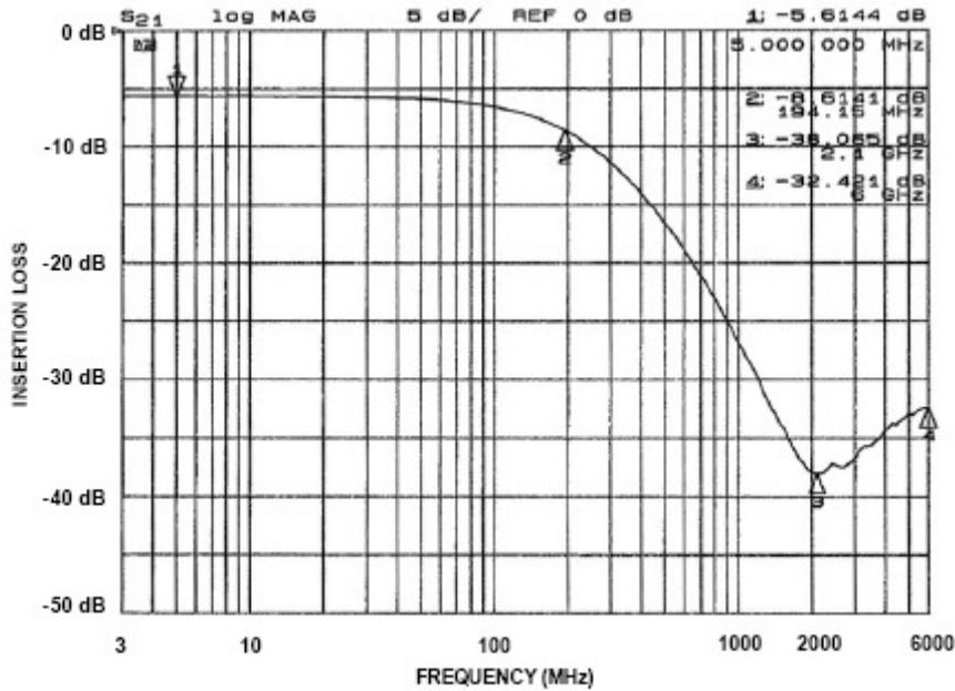
Figure 7. Insertion Loss vs. Frequency (Filter 7 Input – Pin 7 to Pin 10)
