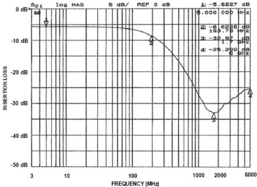
Figure 4. Insertion Loss vs. Frequency (Filter 4 Input – Pin 4 to Pin 13)
