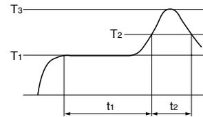
T<sub>1</sub> = 150 to 180°C 302 to 356°F    t<sub>1</sub> = 60s to 120s
