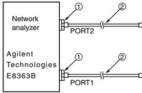
Connect connectors 1 and 2 respectively to PORT 1 and PORT 2. Perform calibration using the 3.5 mm calibration kit (HP85052B).
