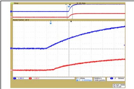
**FIGURE 2-42:** 50 k $\Omega$  – Power-Up Wiper Response Time (1  $\mu\text{s}/\text{Div}$ ).
