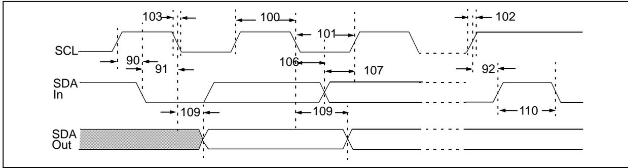
**FIGURE 1-2:** I<sup>2</sup>C Bus Data Timing.
