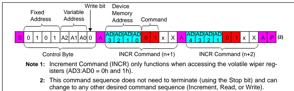
FIGURE 7-7: I<sup>2</sup>C Increment Command Sequence.
