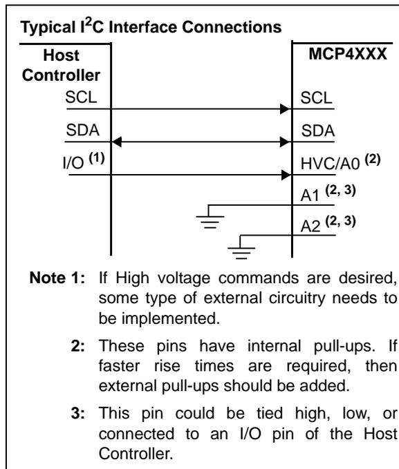
**FIGURE 6-1:** Typical I<sup>2</sup>C Interface Block Diagram.
