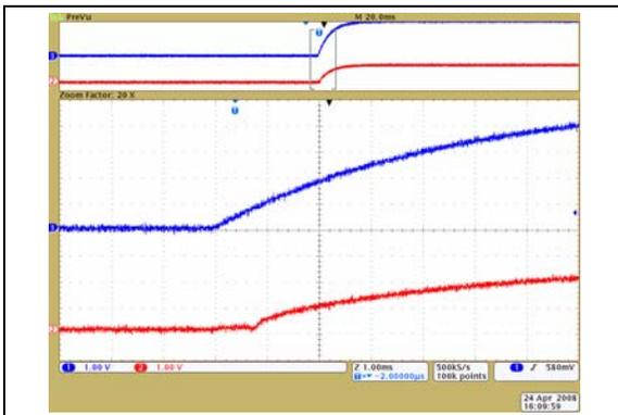
**FIGURE 2-29:** 10 k $\Omega$  – Power-Up Wiper Response Time (1  $\mu\text{s}/\text{Div}$ ).
