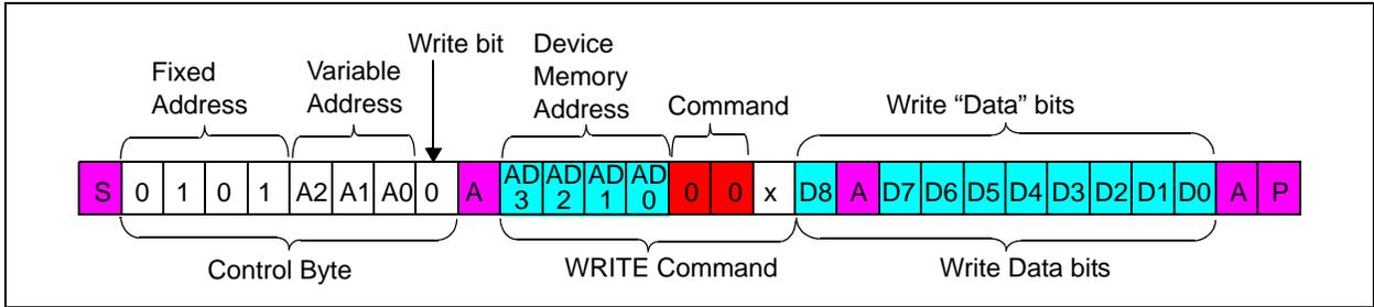
**FIGURE 7-2:** I<sup>2</sup>C Write Sequence.
