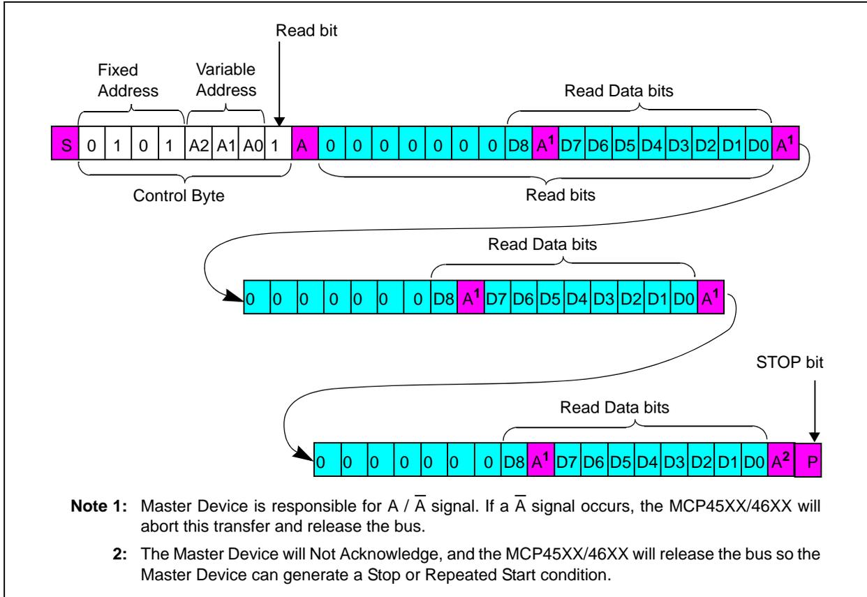
**FIGURE 7-6:** I<sup>2</sup>C Continuous Reads.
