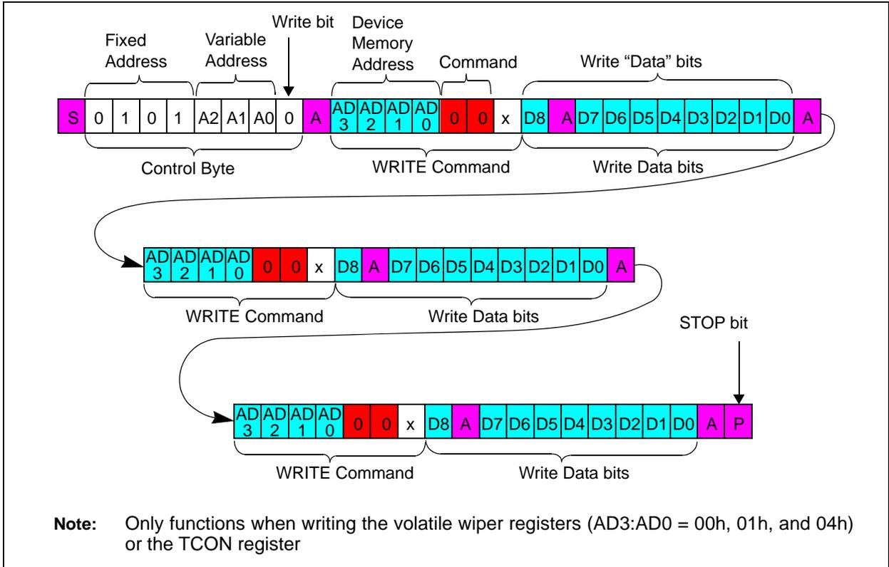
**FIGURE 7-3:** I<sup>2</sup>C Continuous Volatile Wiper Write.
