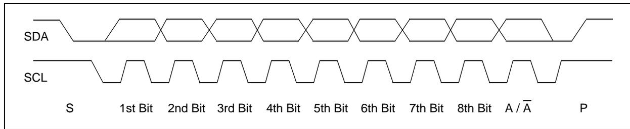
**FIGURE 6-7:** Typical 8-Bit I<sup>2</sup>C Waveform Format.
