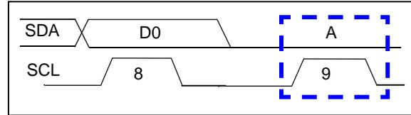
FIGURE 6-4: Acknowledge Waveform.
