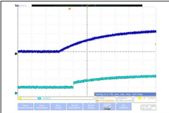
**FIGURE 2-16:** 5 kΩ – Power-Up Wiper Response Time ( $20\ \text{ms}/\text{Div}$ ).
