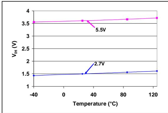
**FIGURE 2-61:**  $V_{IH}$  (SDA, SCL) vs.  $V_{DD}$  and Temperature.
