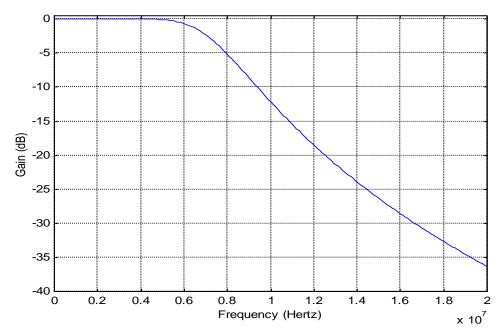
FIGURE 2 THE FREQUENCY RESPONSE OF ANTI-ALIASING FILTER
