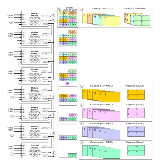
FIGURE 51 INFINITE CASCADE MODE FOR DISPLAY PATH
