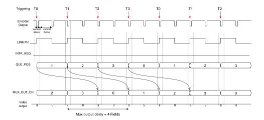
FIGURE 25 THE ILLUSTRATION OF SWITCHING SEQUENCE WHEN QUE\_SIZE = 3, QUE\_PERIOD = 1
