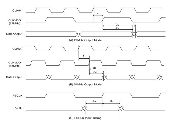
FIGURE 81 CLOCK TIMING DIAGRAM
