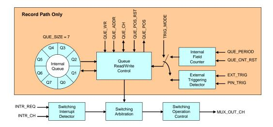
FIGURE 23 THE STRUCTURE OF SWITCHING OPERATION WHEN QUE\_SIZE = 7
