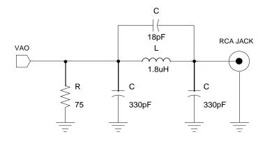
FIGURE 64 EXAMPLE OF RECONSTRUCTION FILTER
