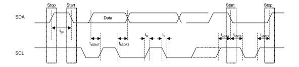
FIGURE 82 SERIAL INTERFACE TIMING DIAGRAM
