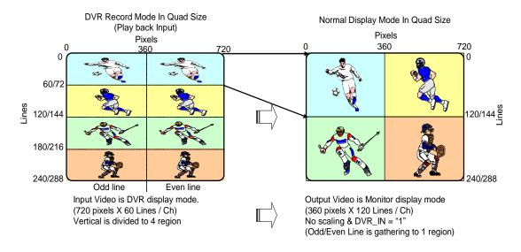
FIGURE 35 THE CONVERSION FROM DVR NORMAL RECORD MODE TO NORMAL DISPLAY MODE
