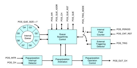
FIGURE 47 THE STRUCTURE OF QUAD\_MUX SWITCHING OPERATION WHEN POS\_SIZE = 7
