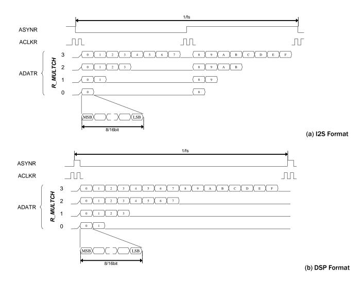
FIGURE 74 TIMING CHART OF MULTI-CHANNEL AUDIO RECORD
