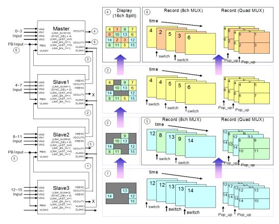
FIGURE 49 THE CASCADE CONNECTION FOR 240 CIF/SEC RECORD MODE
