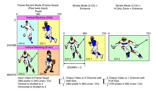
FIGURE 34 THE CONVERSION FROM FRAME RECORD MODE TO FULL IMAGE
