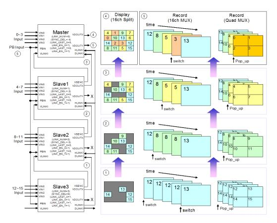
FIGURE 48 THE CASCADE CONNECTION FOR 120 CIF/SEC RECORD MODE
