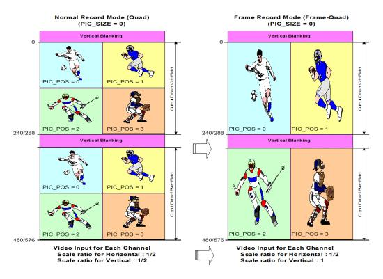
FIGURE 39 THE CHANNEL POSITION AND SIZE CONTROL IN FRAME RECORD MODE
