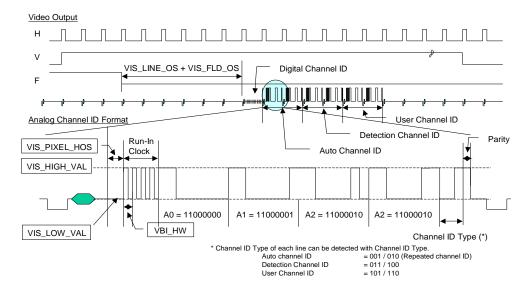
FIGURE 44 ILLUSTRATION OF ANALOG CHANNEL ID
