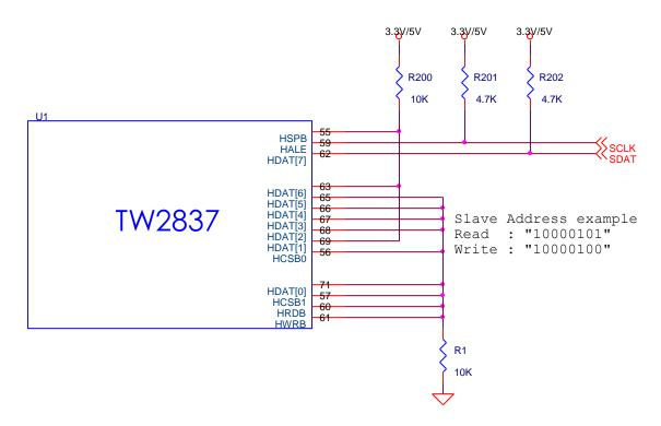
FIGURE 75 THE SERIAL INTERFACE FOR THE CASE OF SLAVE ADDRESS. (READ: "0X85", WRITE: "0X84")
