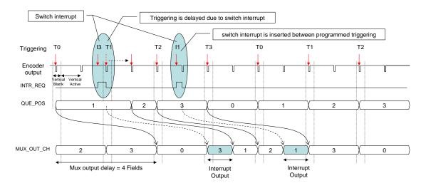
FIGURE 26 THE INTERRUPTED SWITCHING SEQUENCE WHEN QUE\_SIZE = 3, QUE\_PERIOD = 1
