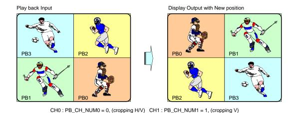
FIGURE 13 THE EFFECT OF AUTO CROPPING FUNCTION
