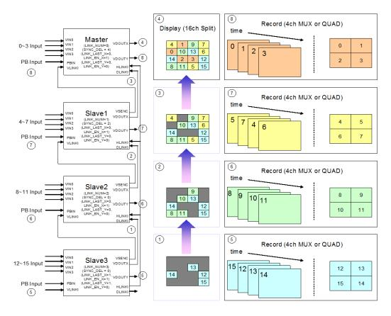
FIGURE 50 THE CASCADE CONNECTION FOR 480 CIF/SEC RECORD MODE
