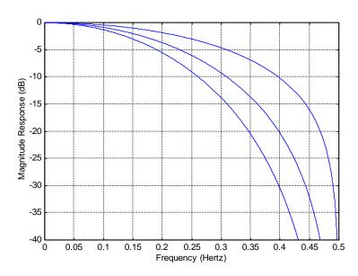
FIGURE 11 THE CHARACTERISTICS OF ANTI-ALIASING FILTER FOR VERTICAL SCALING
