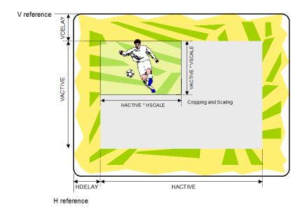
FIGURE 12 THE EFFECT OF CROPPING AND SCALING
