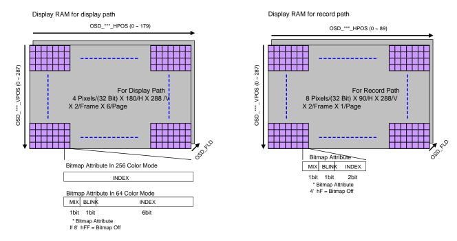
FIGURE 56 THE STRUCTURE OF THE DISPLAY RAM
