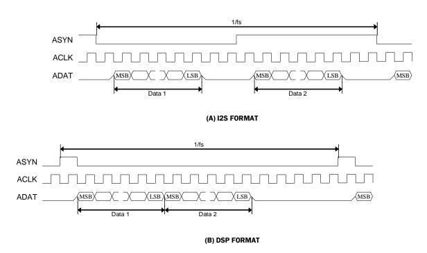
FIGURE 73 TIMING CHART OF SERIAL AUDIO INTERFACE
