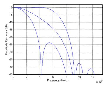
FIGURE 62 CHARACTERISTICS OF LUMINANCE FILTER
