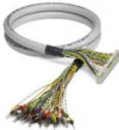
Round cable assembled with a 50-pos. socket strip and an open end. On the open end, the wires are labeled with 1 to 50 and have ferrules, cable length: 6 m
