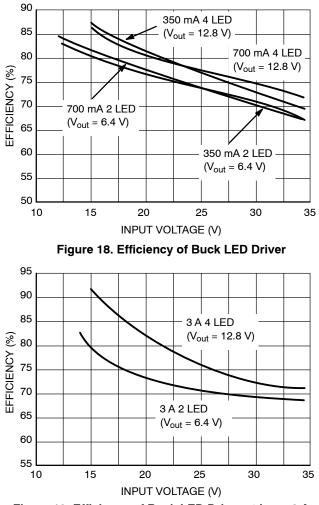
Figure 19. Efficiency of Buck LED Driver at I<sub>out</sub> = 3 A
