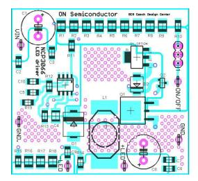
Figure 16. Buck with External Switch Demoboard Layout
