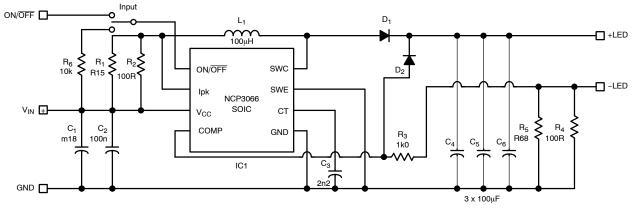
Figure 22. Boost demoboard Application Schematic
