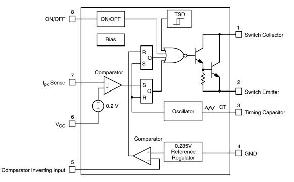
Figure 4. Block Diagram
