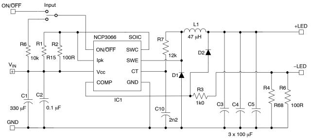
Figure 27. Buck Demoboard Application Schematic
