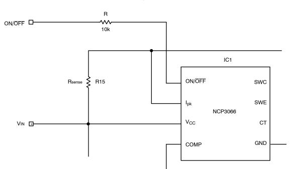
Figure 32. ONOFF Serial Resistor Connection
