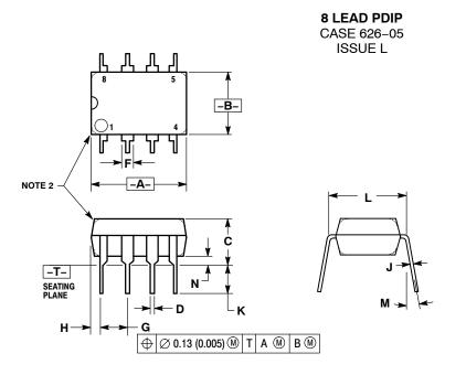
NOTES: 1. DIMENSION L TO CENTER OF LEAD WHEN FORMED PARALLEL. 2. PACKAGE CONTOUR OPTIONAL (ROUND OR SQUARE CORNERS). 3. DIMENSIONING AND TOLERANCING PER ANSI Y14.5M, 1982.
