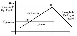
Figure 13. Current Sense Waveform
