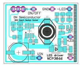
Figure 23. Boost Demoboard Layout
