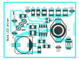
Figure 28. Buck Demoboard Layout
