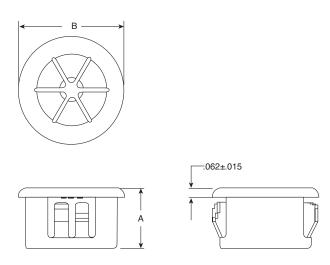
Nylon "ALL-FIT" Adjustable Bushings are designed to protect wire, cable, tubing, or irregular shaped items from sharp, unfinished edges. The specially designed, resilient multiple supports absorb shock and vibration and adjust to accept various diameters and shapes. The All-Fit Bushing is equipped with multiple locks to positively snap in panel thicknesses ranging from 1/32" to 1/8". Molded in heat stabilized nylon UL94V2 black.
