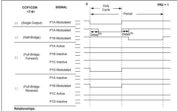
Note 1: Dead-band delay is programmed using the PWM1CON register (Section 15.4.6 "Programmable
