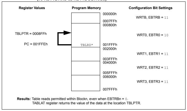
FIGURE 22-9: EXTERNAL BLOCK TABLE READ (EBTRn) DISALLOWED (48-KBYTE AND 64-KBYTE DEVICES)
