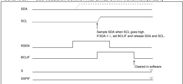
FIGURE 16-30: BUS COLLISION DURING REPEATED START CONDITION (CASE 2)
