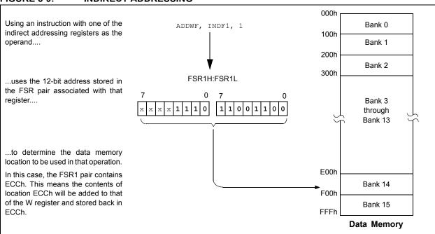
The PLUSW register can be used to implement a form of indexed addressing in the data memory space. By manipulating the value in the W register, users can reach addresses that are fixed offsets from pointer addresses. In some applications, this can be used to implement some powerful program control structure, such as software stacks, inside of data memory.
