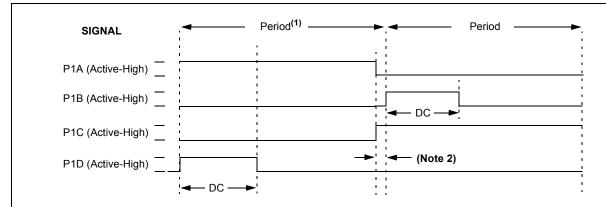
Note 1: The direction bit in the CCP1 Control register (CCP1CON<7>) is written any time during the PWM cycle. 2: When changing directions, the P1A and P1C signals switch before the end of the current PWM cycle at intervals of 4 Tosc, 16 Tosc or 64 Tosc, depending on the Timer2 prescaler value. The modulated P1B and P1D signals are inactive at this time.
