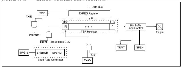
FIGURE 17-4: ASYNCHRONOUS TRANSMISSION
