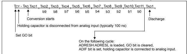
FIGURE 18-5: A/D CONVERSION TAD CYCLES (ACQT<2:0> = 010, TACQ = 4 TAD)
