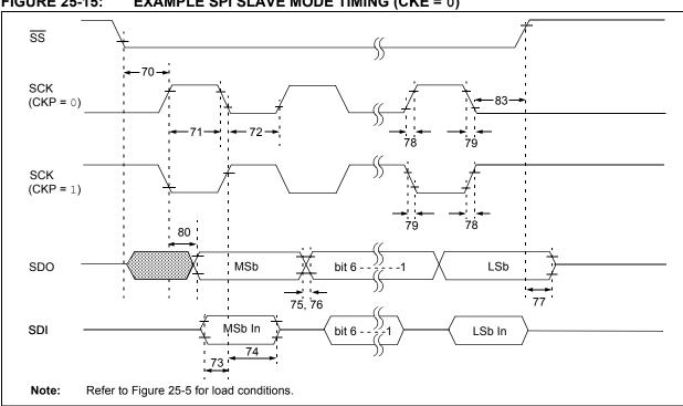
FIGURE 25-15: **EXAMPLE SPI SLAVE MODE TIMING (CKE = 0)**
