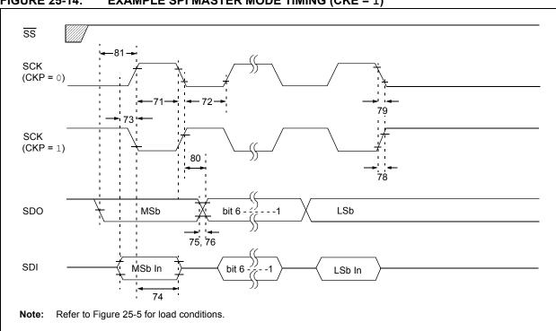
FIGURE 25-14: EXAMPLE SPI MASTER MODE TIMING (CKE = 1)
