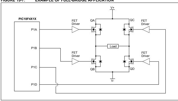
FIGURE 15-7: EXAMPLE OF FULL-BRIDGE APPLICATION
