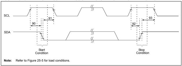
TABLE 25-20: MASTER SSP I<sup>2</sup>C™ BUS START/STOP BITS REQUIREMENTS
