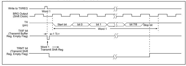
FIGURE 17-5: ASYNCHRONOUS TRANSMISSION (BACK TO BACK)
