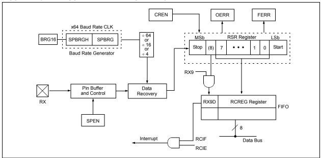
FIGURE 17-7: ASYNCHRONOUS RECEPTION
