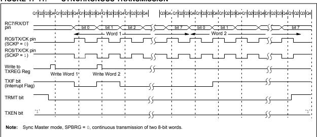
FIGURE 17-12: SYNCHRONOUS TRANSMISSION (THROUGH TXEN) RC7/RX/DT pin bit 0 bit 2 bit 1 bit 7 RC6/TX/CK pin Write to TXREG reg TXIF bit TRMT bit TXEN bit
