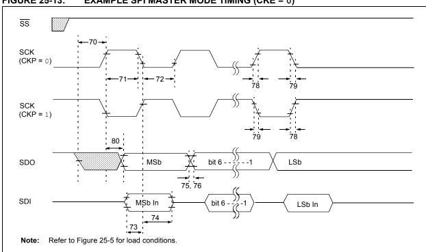
FIGURE 25-13: EXAMPLE SPI MASTER MODE TIMING (CKE = 0)
