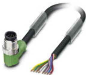
Sensor/actuator cable, 8-position, PUR halogen-free, black-gray RAL 7021, Plug angled M12, coding: A, on free cable end, cable length: 1.5 m
