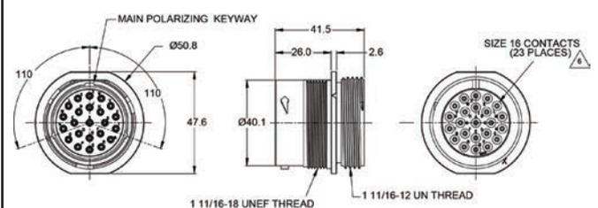
Standard and reverse terminal genders allows for custom polarization
