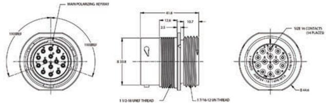
*Standard and reverse terminal genders allows for custom polarization*
