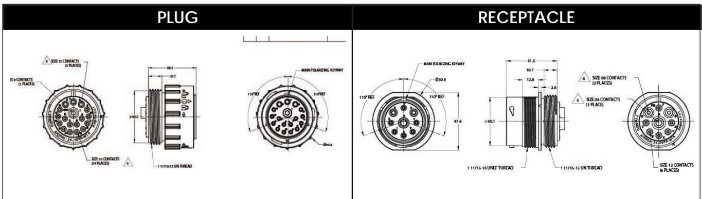
Standard and reverse terminal genders allows for custom polarization
