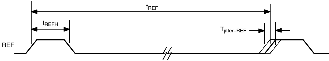
Figure 5. REF Input Timing Diagram
