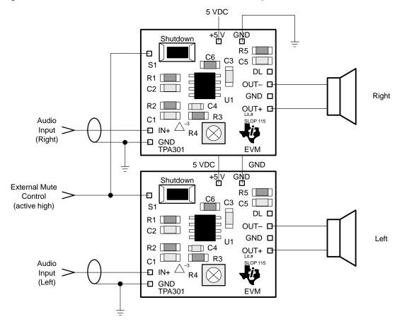
Figure 3–8. TPA301 EVM Connected for Stereo BTL Output
