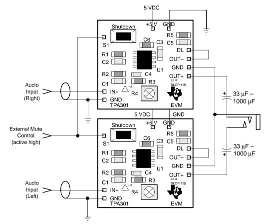
Figure 3–9. TPA301 EVM Connected for Stereo Single-Ended Output
