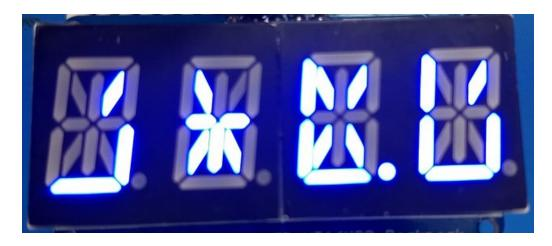
You might notice the display turns on to a 'jumbled' collection of random LEDs. Don't worry! The display isn't broken, right now the module that controls it doesn't clear the display state on startup so you might see noise from random memory values.
