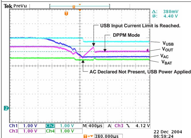
Figure 10. Remove AC – PWR XFER to USB
