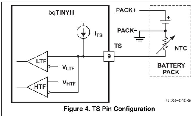
Figure 4. TS Pin Configuration
